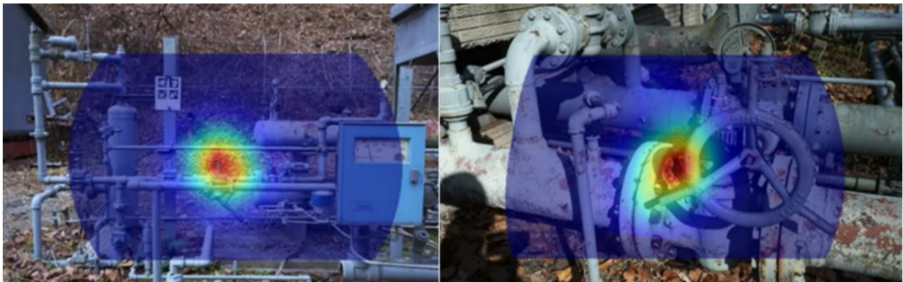
Figure 9. Examples of component-level emission source detection in oil and gas facilities recorded from distances of 3 meters and 1 meter.
