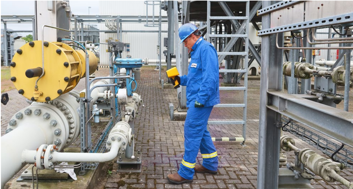
Figure 10. Scanning equipment and components with Xplorobot Laser OGI device.
