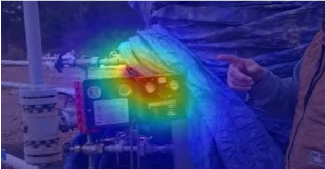
Figure 11. Detection of the emission (column-integrated concentration above 500ppm-m) and visualization of the emission otherwise not visible to the naked eye by the Xplorobot Laser OGI device.
