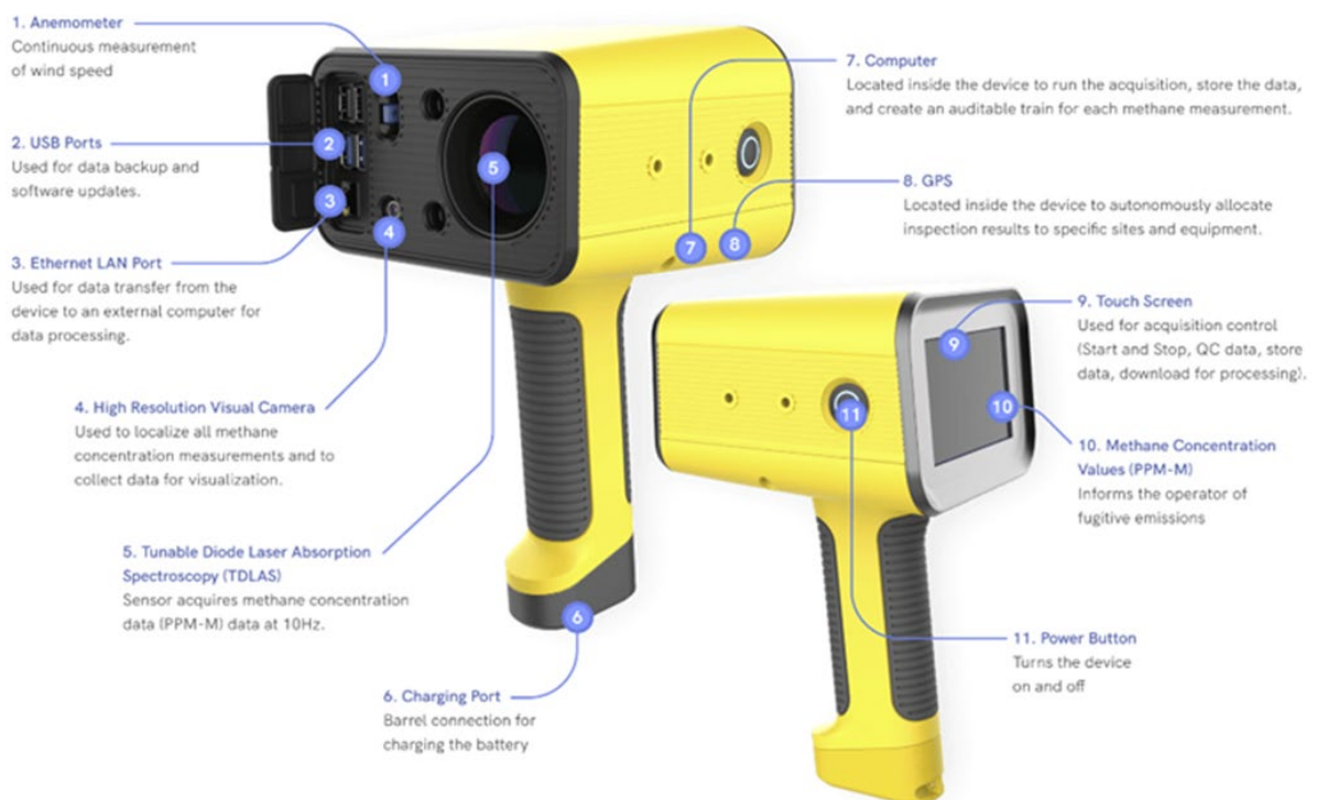
Figure 1. Xplorobot Laser OGI device and its elements
