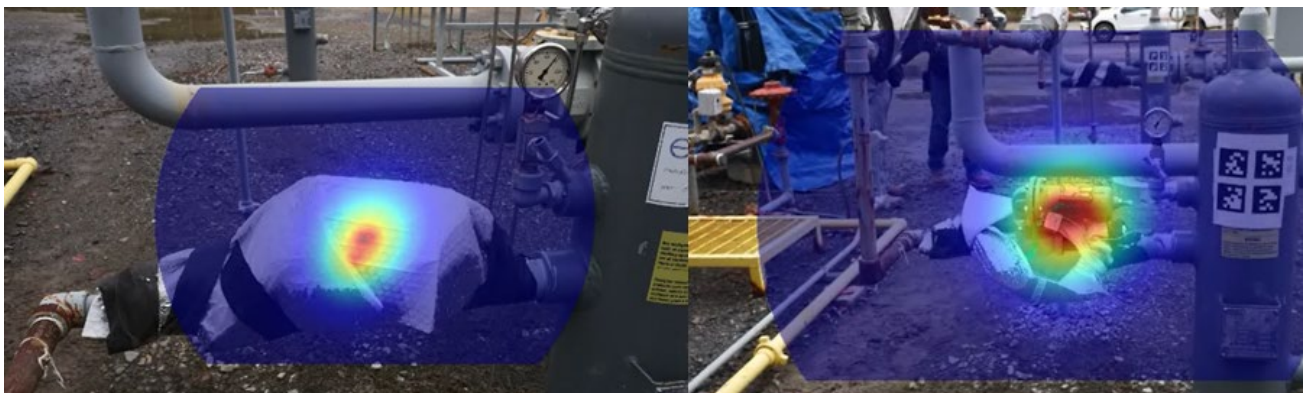
Figure 7. Emissions were detected under a bubble wrap, and the recording on the regulator after the wrap was removed.
